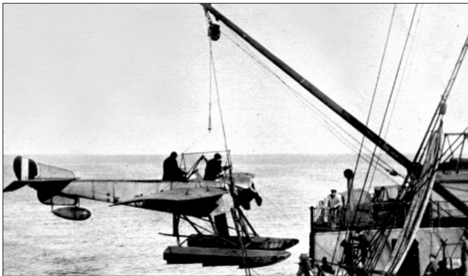
Nieuport XH seaplane in profile, with derrick. HMS Anne , February 1916. (Courtesy ARDHAN)
