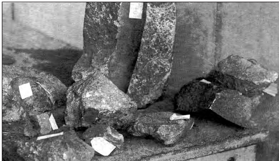
Turkish 'Old' type shell fragments recovered from HMS Agamemnon 25 February 1915. Note the large size of the fragments, their thick walls, and reduced space for the bursting charge. From Dardanelles: a Midshipman's Diary
