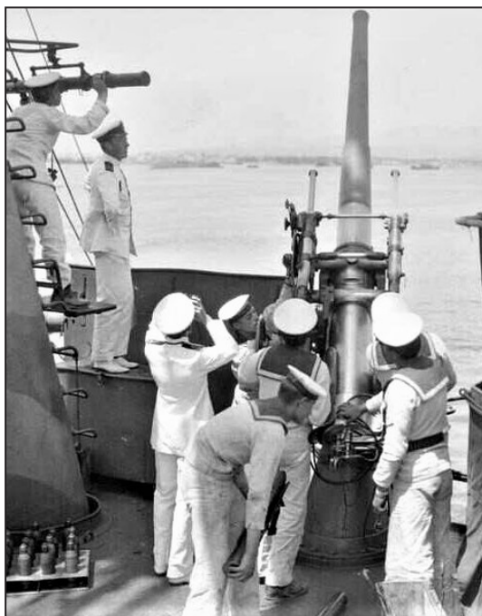
HMS Agamemnon 12-pdr (1916). Note that the gun seen here is demonstrating high-angle anti-aircraft fire.
