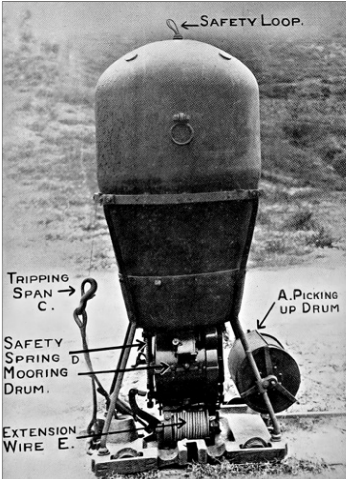
German manufactured Carbonit Co. contact mine of the type encountered in this action (from The Mitchell Report , 1919). NB: the mine's horns are not shown here.
